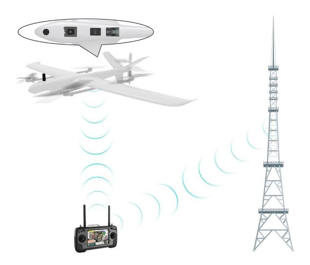
Run Mission Planner on SIYI handheld ground station and connect SIYI handheld ground station to Internet. Go to "SETUP – RTK / GPS Inject – NTRIP".
